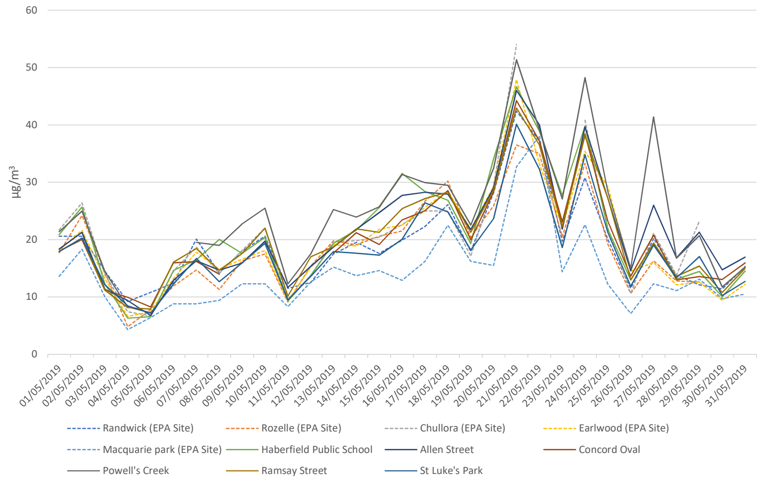
Comparison of WestConnex M4 sites with EPA Sites PM 10 24hr average May 2019
